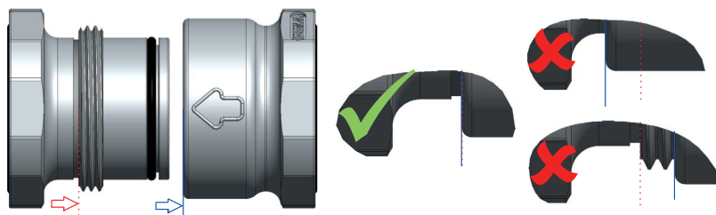
Fig. 17: Verifying the alignment
